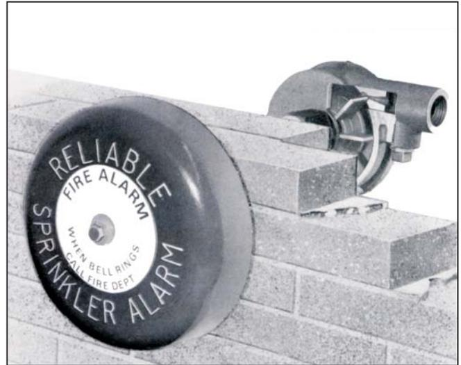
The Reliable Model C Mechanical Alarm, also called a water motor and gong, is the hydro-mechanical alarm of Reliable Wet and Dry Pipe Automatic Sprinkler Systems. Usually mounted on an outside building wall and energized by water flowing from the alarm (wet) or dry pipe valve, it automatically sounds a continuous piercing alarm when the sprinkler system operates to extinguish a fire.
